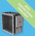
In case of an explosion, blast dampers protect people and equipment. Without proper blast protection, a blast wave could penetrate the building through air intakes and outlets. Blast dampers close automatically when the blast wave hits them. Halton blast dampers are available as ATEX-approved.
