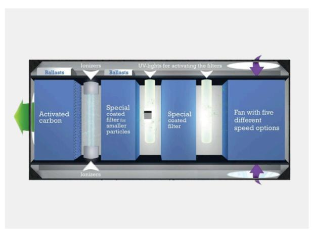
• Four stage filtration includes: Bi-polar ionization, UVGI light, filtering, photo-catalytic oxidation. Note: patented process
