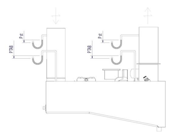
$\Omega P_{st}$  = Static pressure loss
