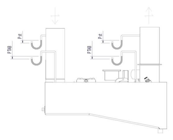
$\Omega P_{st}$  = Static pressure loss
