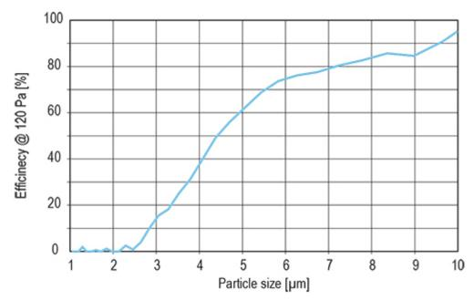
Mechanical filtration is recommended to be used in hoods with low utilization rate and cooking process producing mainly large grease particles (> 8 microns), e.g. food prepared with gas fryers, griddles and broilers (source ASHRAE).
