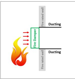
Picture 1. Fire Damper preventing the fire from spreading.
