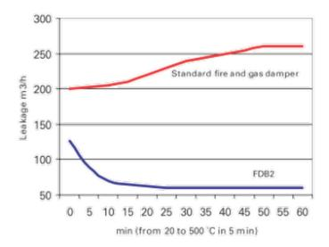
Graph 1. Leakage rate of Halton gastight fire damper in high heat.
